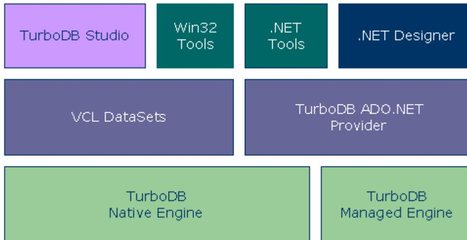
At the basis, there are two database kernel implementations. One is for native Win32 and therefore compiled to machine language, the other is for .NET and consists of 100% managed code. When programming on the .NET platform, you can use either one with different advantages:
